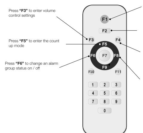
"F1" switches to time mode when a count down /up is in progress. Press "F1" to exit setting mode without saving
