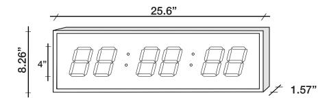
**NOTE:** Model XL-46R-100 is a plug-in digital clock. A small battery is included in the clock for backup purposes in order to maintain clock functions in the background. The battery will however not illuminate the display. The clock will remain on time when power resumes. Model XL-46R-100 is exclusively operated with the remote control supplied with the clock.
